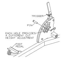
The two holes at the front of the quadrant are for 1-1/2" and 1-3/4" cut heights.
